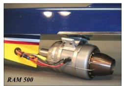
possible. In fact, a neatly-done notch in the rear edge of the boat tail may allow you to move the turbine forward an extra half inch or more. Use four #6 x 1" stainless steel sheet metal screws to hold the aluminum mount and thrust wedge in place.
